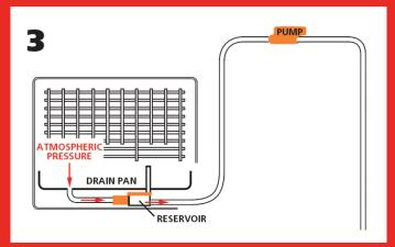
Water level in the reservoir has now receded enough to drop the float, deactivating the pump. However, the weight of the water in the discharge hose plus atmospheric pressure at the drain pan outlet forces the water remaining in the intake hose to continue flowing out through the pump until the reservoir intake hose, pump and discharge hose are completely empty, at which point the siphoning stops.
