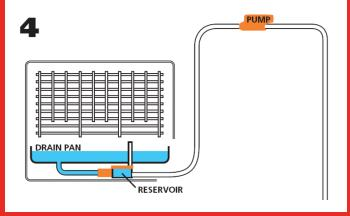
As the evaporator produces more condensate, the drain pan again fills up with water which flows into the reservoir. Since the intake hose is filled with air again, the cycle repeats itself.
