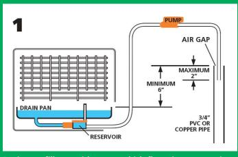
Drain pan fills up with water which flows into reservoir. Intake hose between reservoir and pump is empty i.e. filled with air.
