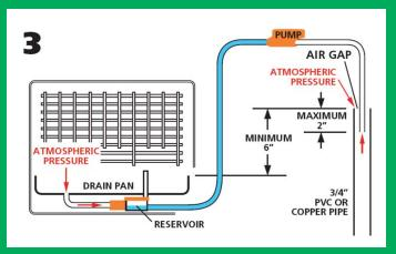
Water level in the reservoir has now receded enough to lower the float which deactivates the pump, however, since an air gap is in the discharge hose, atmospheric pressure is equalized at both ends of the hose system so the siphoning effect cannot occur and THE INTAKE HOSE REMAINS FILLED WITH WATER.
