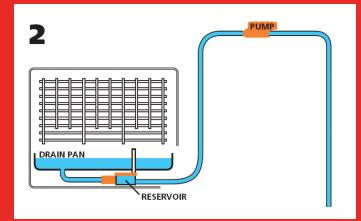
Rising water lifts the float, activating the pump, which self primes by sucking water from reservoir. During this period the pump is operating hot and dry and will click loudly. Once the air in the intake hose has been purged, water entering the pump cools and lubricates, so that the clicking noise becomes a low hum. Water flows through the pump and out the discharge hose.
