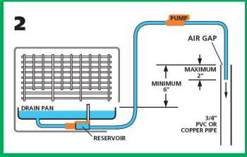
Rising water lifts float, activating the pump, which self primes sucking water up from reservoir. During this period the pump is operating hot and dry and will click loudly. Once the air in the intake hose has been purged, water entering the pump cools and lubricates it so that the clicking noise becomes a low hum. Water flows through the pump and out the discharge hose.
