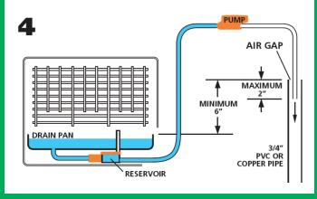
The drain pan again fills up with water which flows into the reservoir and activates the pump. THE INTAKE HOSE IS ALREADY FILLED WITH WATER so no air is sucked in, and the pump is immediately cooled and lubricated. No clicking noise is heard.
