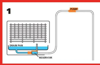
Drain pan fills with water which flows into reservoir. Intake hose between reservoir and pump is empty i.e. filled with air.
